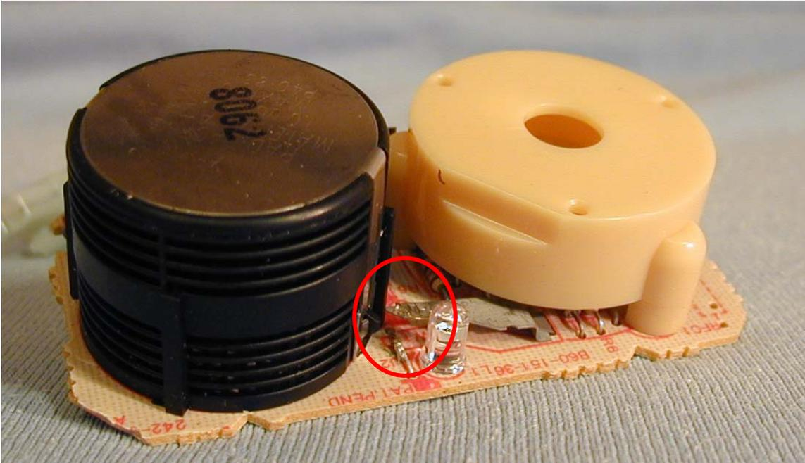
By looking at the front and back of the board, I located the corresponding ends of the “switch”, and soldered a wire across to make permanent contact.
