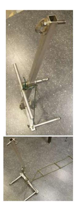
Detail of the riser-to-base join (bottom). The riser is 30x30mm, 2mm thick square aluminium; the top part of the riser is 25x25x2 to fit snugly inside. The bottom frame is also 30x30x2mm.
